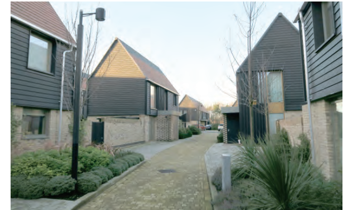
The careful orientation of terraces and placement of windows can ensure that both privacy and high density is achieved.
